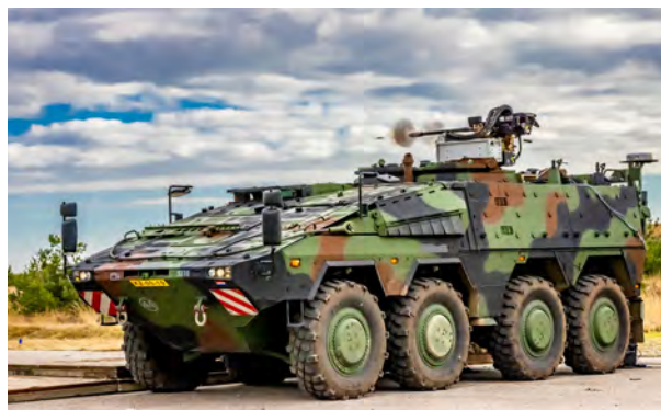
EOS R400S Dual Weapon System firing off a Royal Netherlands Army 8 x 8 Boxer Combat Reconnaissance Vehicle
