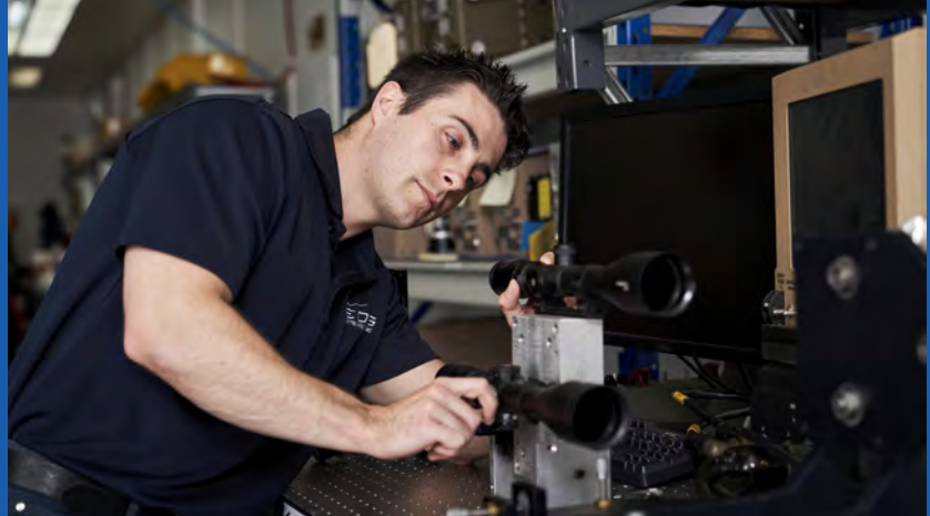
Paul Costigan calibrates an optical table used in the production of EOS sensor units
