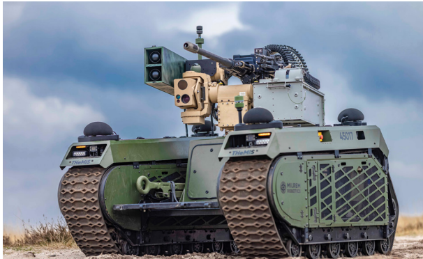
The EOS R400 RWS in CUAS and anti-tank configuration on the Milrem TheMIS uncrewed ground vehicle (UGV)
