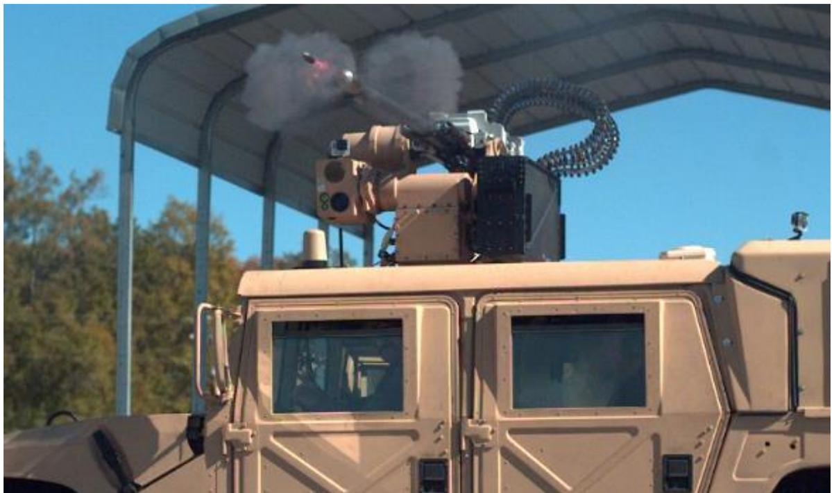
High speed photograph of M230LF firing from R-400S on HMMWV
