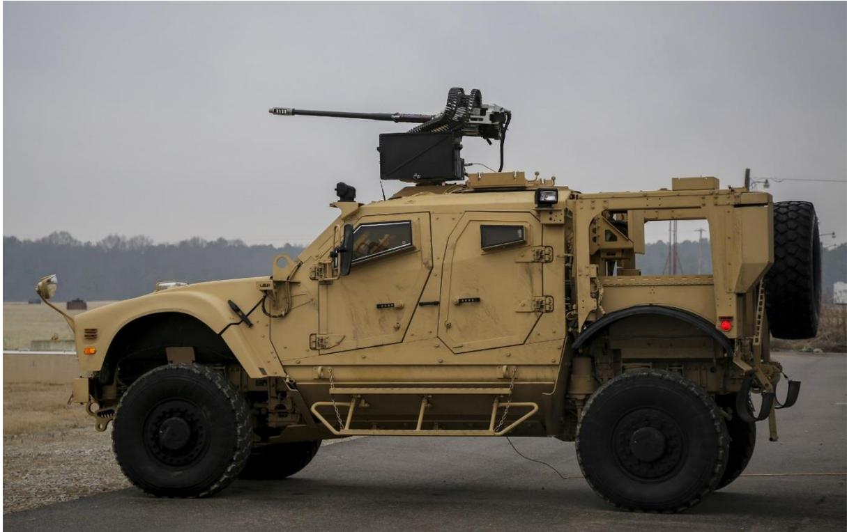
R-400S with ATK M230LF 30mm cannon mounted on Oshkosh M-ATV
