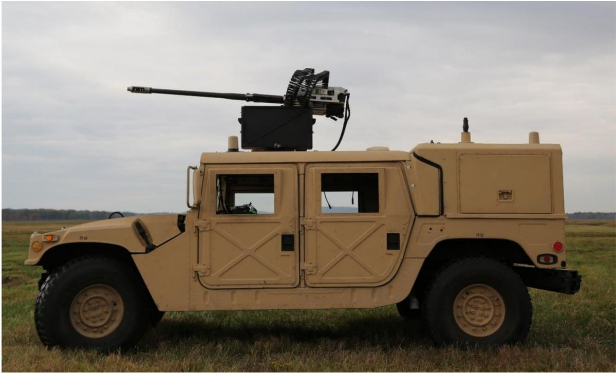
R-400S with ATK M230LF 30mm cannon mounted on HMMWV
